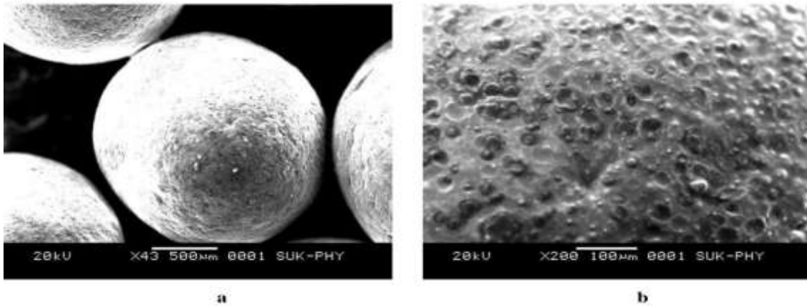
Figure 5.9.2 Scanning electron microscopy of (a) external and (b) surface morphology of drug loaded floating beads (F1)
